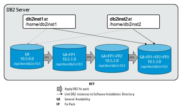
The diagram shows a DB2 server with two instances. The DB2 instances point to the DB2 Software Installation Directory that is updated over time with subsequent DB2 server fix packs.
