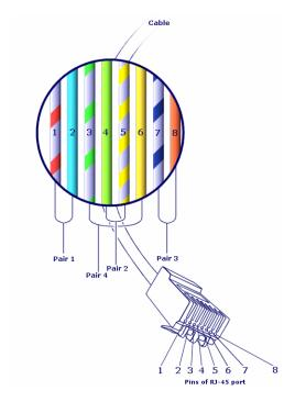
If we take the **RJ-45** connector, each pin is associated with a wire having a given color and a given duty:
