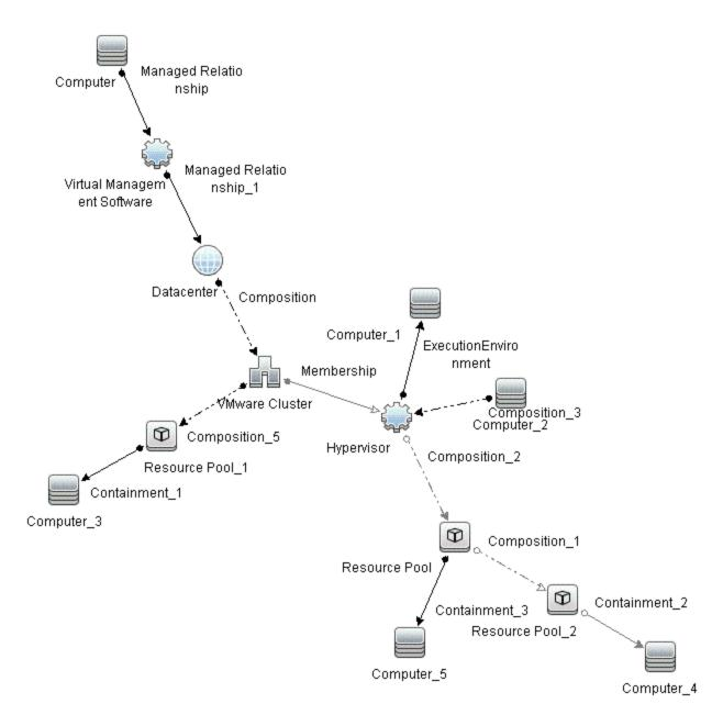
• vMA\_Infrastructure: This view shows the vMA, virtual management software and relation between vMA and virtual machines. vMA collects the data for hosts and virtual machines.
