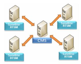
RTSM is the operational storage of BSM. Configuration items (CIs) discovered by different BSM data sources are reconciled and stored in the RTSM.
