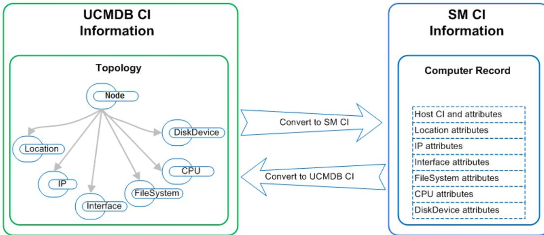
The above figure shows the correlation between the UCMDB topological model and its representation of the Computer Instance together with its parallel representation in SM. The SM computer CI contains all of the UCMDB information that is passed through the integration.
