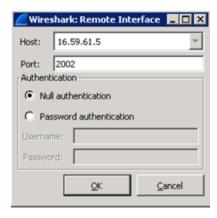
7. Click **OK** to add the remote interface. The new remote interface appears in the Remote Interfaces tab of the Interface Management window.
