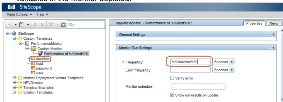
**Figure 27: SiteScope: enter variable to associate with template**
