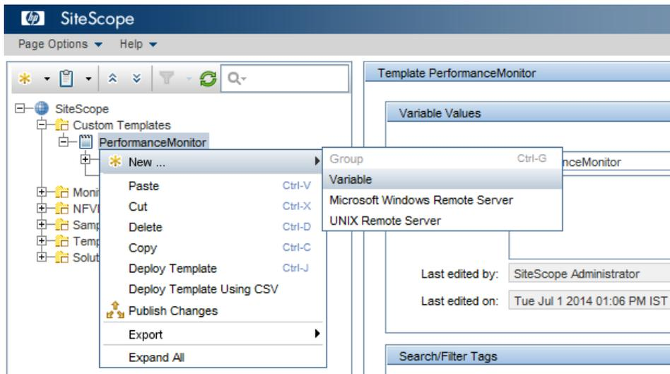
**Figure 25: SiteScope: new Variable**
