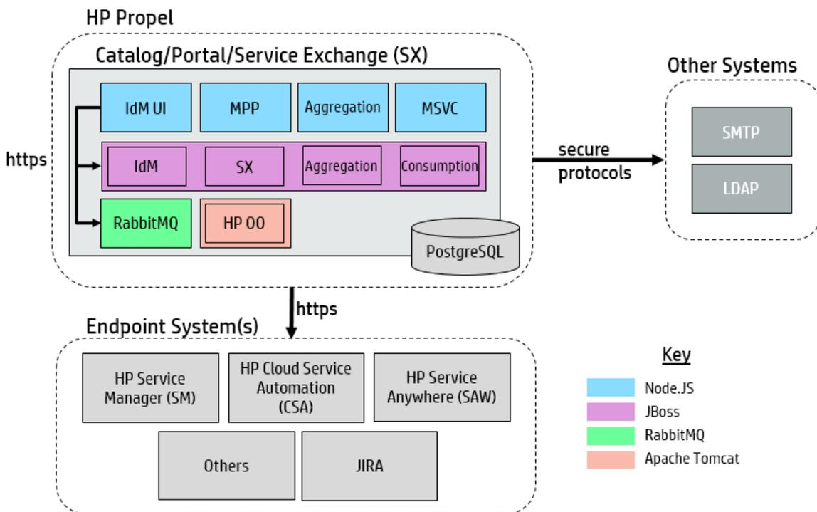
Drill down to the internal communications inside the HP Propel machine.
