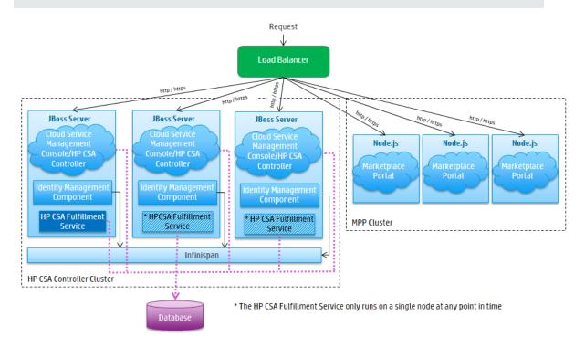
The cluster uses a load balancer to distribute requests among any number of nodes. The load balancer (internal or external) listens for HTTP/S requests from standard interface clients. Nodes are transparent to users and users access only the URL to the load balancer. The load balancer forwards HTTP/S requests to one of the other nodes.
