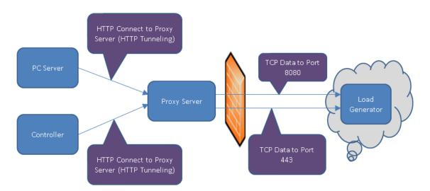
The communication is initiated from the Performance Center server and the Controller to the defined proxy server. An HTTP Tunnel is used as a means for communicating from the Performance Center server and the Controller to the proxy server. The proxy server then runs over the firewall and transfers the data to the cloud-based load generator, going through the TCP ports.
