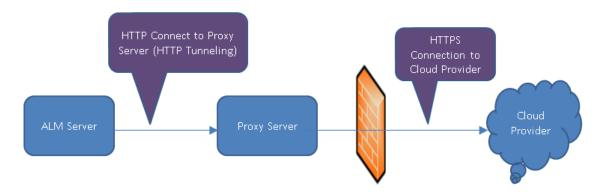
The communication is initiated from the ALM server to the defined proxy server using HTTP tunneling. The proxy server then runs over the organization's firewall and transfers outgoing requests to the cloud provider.
