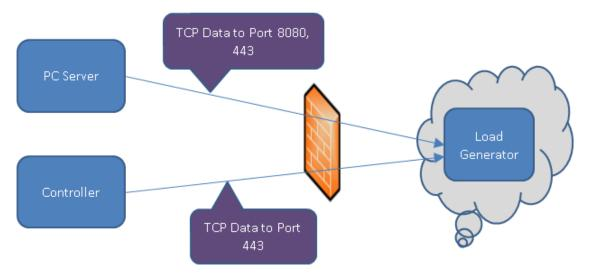
The communication is initiated from the Performance Center server and the Controller over a firewall to the cloud-based load generator. Data is transmitted through TCP (Transmission Control Protocol) using ports. The ports are opened for outgoing requests. The ports can be reconfigured.
