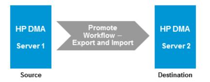
This is useful, for example, when you want to copy a workflow that has been validated in your test environment onto an HP DMA server in your production environment.
