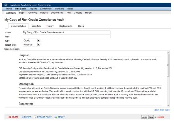
A workflow consists of a sequence of **steps**. Each step performs a very specific task. Each step includes a documentation panel that briefly describes its function.
