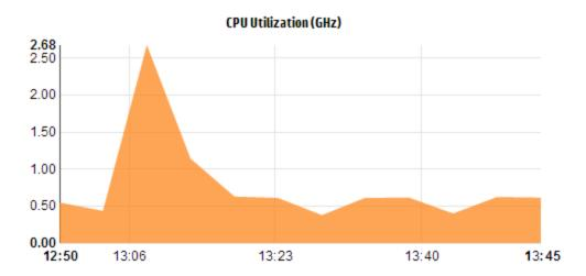
In the preceding figure, the graph shows the CPU utilization for the selected VM. The vertical axis shows the utilization specific to the VM in GHz.
