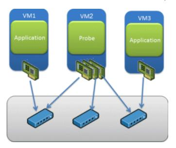
There are two entities in VMware—a virtual switch and portgroups. By default, a guest operating a system's virtual network adapter only receives frames specific for that adapter. Placing the guest adapter in promiscuous mode causes it to detect all frames passed through the virtual switch that are allowed under the VLAN policy for the associated portgroup.
