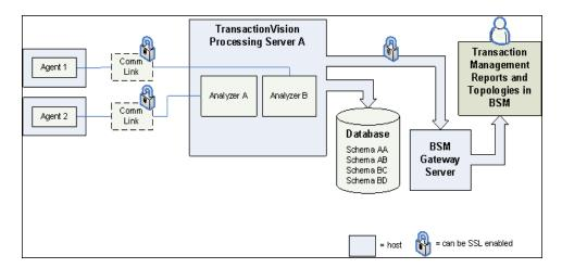
The following sections describe how to enable SSL on the TransactionVision Processing Server to the Gateway Server pathway (right side of the diagram), and on the communication link data pathway (left side of the diagram), which is dependent on the type of agent and message middleware provider.
