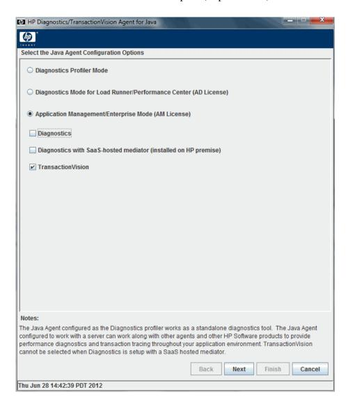
These options set the value of the **active.properties** property in the **etc/probe.properties** file to **TV** mode.
