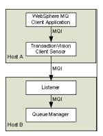
In general, applications that make use of WebSphere MQ client binding will communicate with a "listener" process (also known as the channel responder) that runs on the same host as the targeted queue manager. All WebSphere MQ activities (that is, MQI calls) are forwarded to and processed by the listener program, which in turn issues the appropriate MQI calls to the corresponding queue managers on behalf of the client applications.
