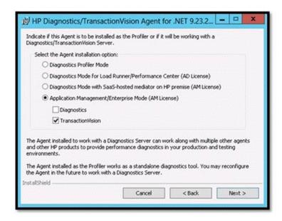
These options set the value of the probe\_config.xml <modes> element to tv mode. The mode value in the probe\_config.xml <modes> element is also used in determining usage against the license capacity. Agents in AM mode are always counted against the AM license capacity.
