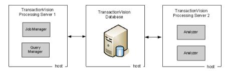
➤ One Processing Server for the Job Manager, the Query Manager, and one instance of the Analyzer, one Processing Server for another Analyzer:
