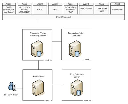
**Note:** Each TransactionVision Processing Server contains an embedded database that can be used in place of the TransactionVision database for POC or other testing purposes.
