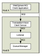
In this case, the agent is deployed on the host where the listener process and queue manager reside. Instead of direct monitoring of the client application, the agent monitors the listener program instead.
