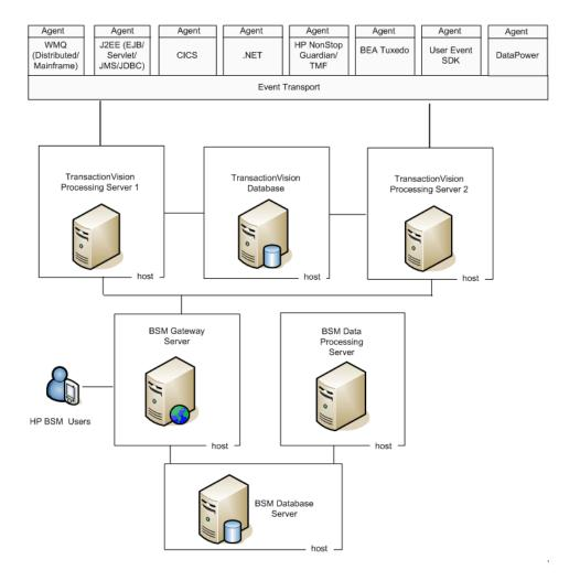
The database used by TransactionVision is separate from the database used by BSM, and must be installed on a host that is accessible from every TransactionVision Processing Server.
