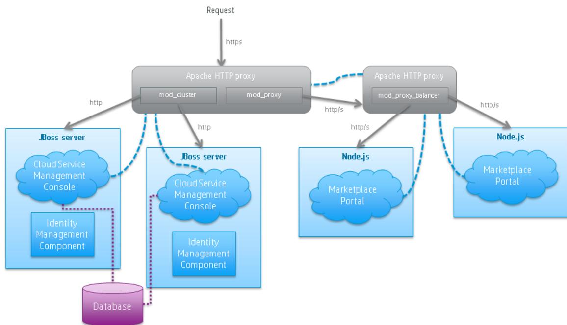
The cluster uses a Web server to distribute requests among any number of nodes and can be useful to an organization that already uses a standard Web server within its network infrastructure. The Web server (internal or external) listens for HTTPS requests from standard interface clients. Nodes are transparent to users and users access only the URL to the Web server. The Web server forwards HTTP requests to one of the other nodes.
