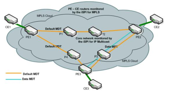
Monitoring the network using the NNM iSPI for MPLS and NNM iSPI for IP Multicast
