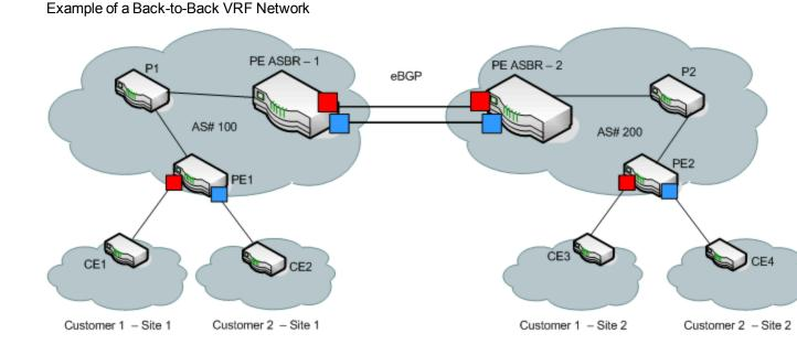
The NNM iSPI for MPLS discovers CE nodes that are located outside the MPLS VPN Network. The NNM iSPI for MPLS detects and manages all the nodes participating in the back-to-back VRF setup. You can monitor the connectivity between the PE node residing in the MPLS VPN Network, the IP addresses and AS#s of carrier service provider network, and geographically dispersed CE nodes residing within the client sites. The NNM iSPI for MPLS helps you view:
