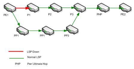
In the example, the fault occurred at Provider Edge router (PE1) and the LSP got re-routed to alternate Provider routers (PP1-PP2-PP3). In this case, a **Re-route** incident is generated for the LSP originating from PE1.
