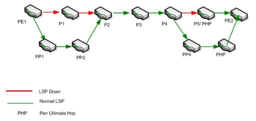
The re-route incident is generated only the first time, in this case the LSP is first Re-routed at PE1 and then again at P4. The re-route incident is generated at PE1.
