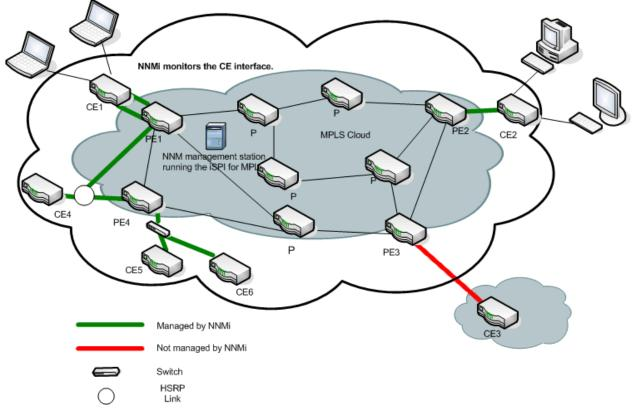
Example of the PE - CE connectivity on the network
