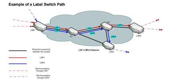
In the example above, there are two LSPs passing through an MPLS cloud. The first one connects the the Edge Routers LER1 and LER3 by passing through P Routers (P1 and P2). The second originates from edge router LER1 and passes through the P Routers P1 and P2, and ends at Edge Router LER2. In this example, LSP1 is mapped to two services and LSP2 is mapped to one service.
