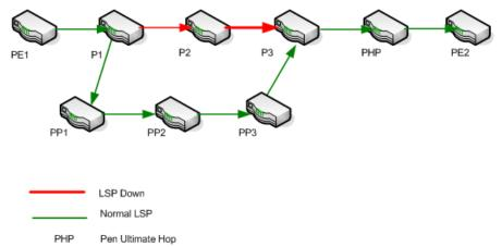
In the example, the fault occurred at Provider router (P1) and the LSP got re-routed to alternate Provider routers (PP1-PP2-PP3). In this case, a Re-route incident is generated for the LSP originating from P1.
