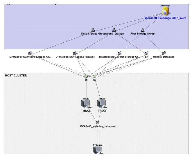
The dotted lines show the replication path of each database and storage groups against the passive node.
