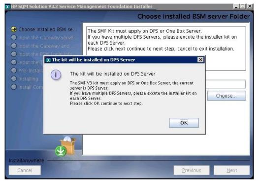
6. If the SMF 2.3 or above version kit is already installed, the following dialog box will appear, click ok to exit install application, and then uninstall the current exist SMF Kit before strating a new install.
