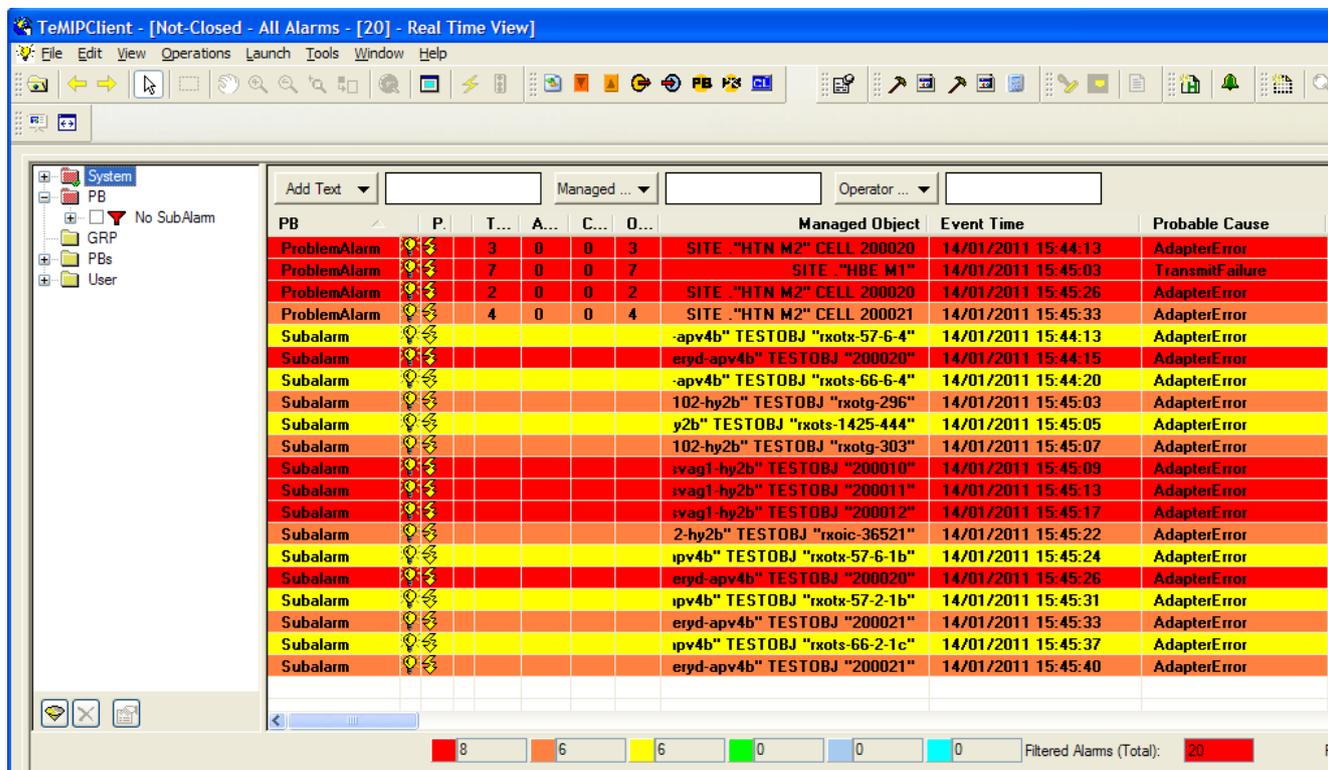
Figure 3: Filter pattern [No SubAlarm] deactivated: 20 alarms displayed
