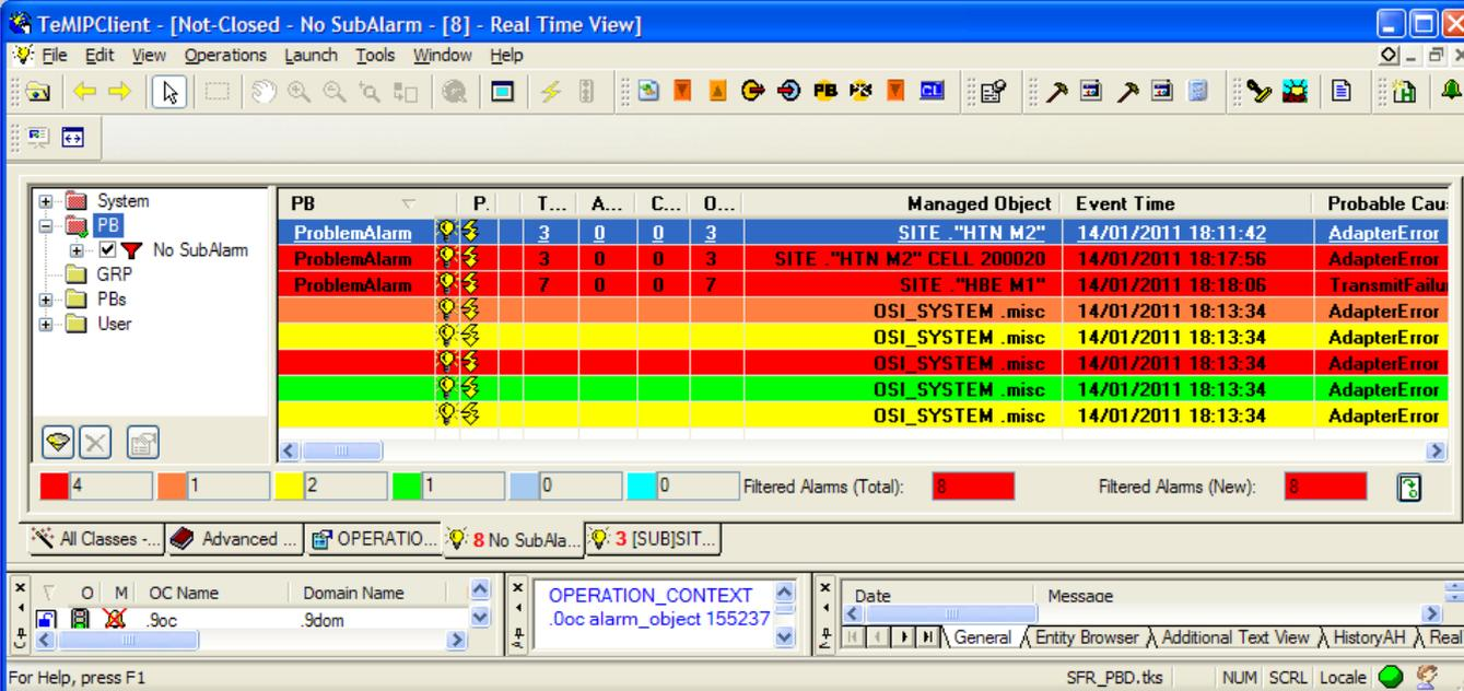
The screenshot shows the TeMIPClient interface with a table of alarms. The table has columns for PB, P, T, A, C, O, Managed Object, Event Time, and Probable Cause. The table contains several rows of data, including ProblemAlarms and OSI\_SYSTEM .misc entries.
