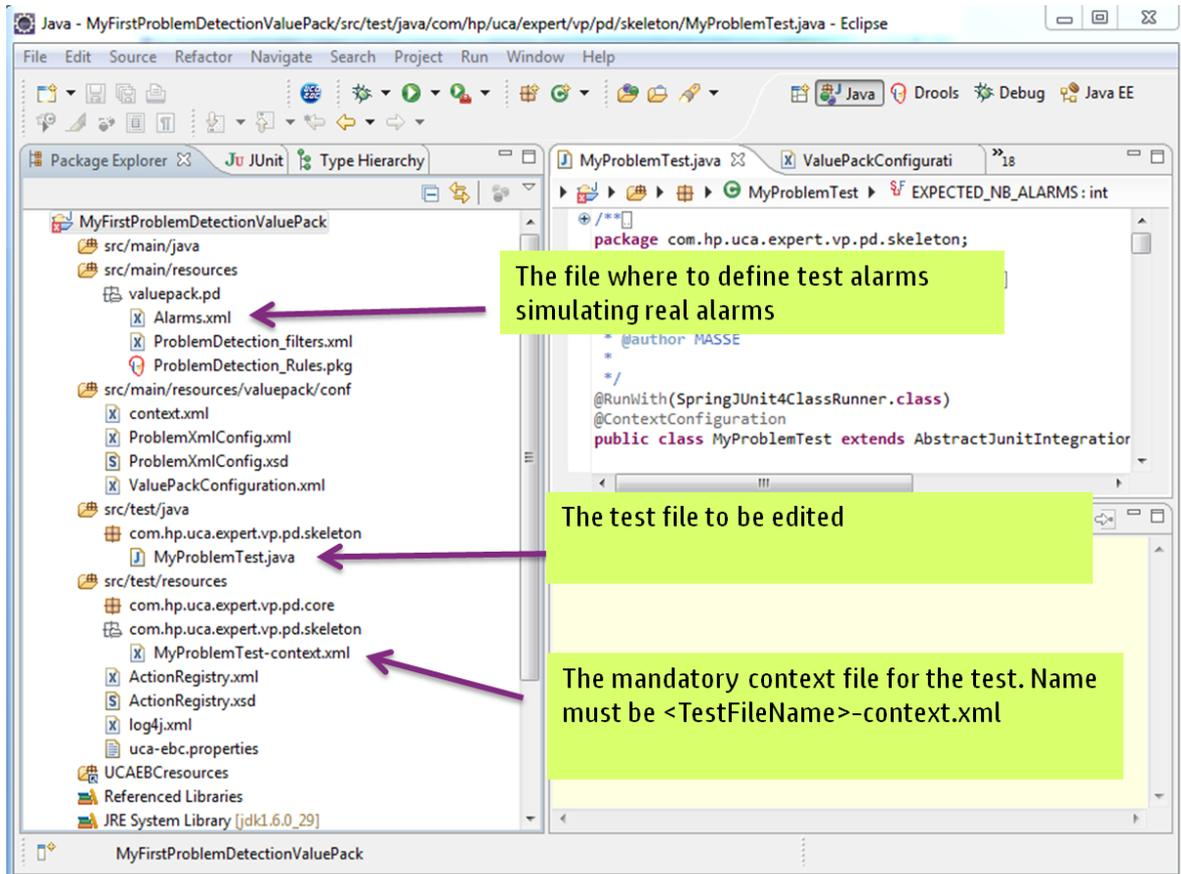
Figure 14 - Files to modify to create a JUnit test
