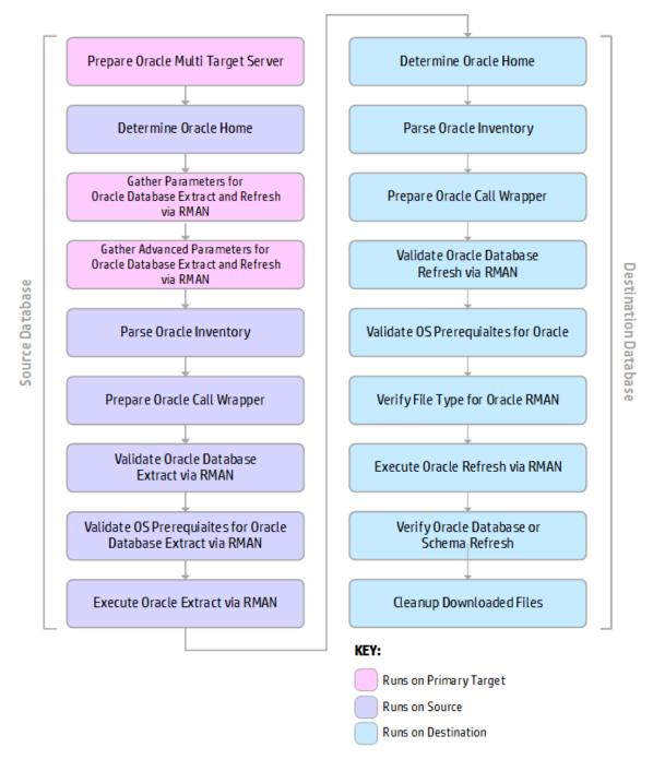
The first step of the workflow, Prepare Oracle Multi Target Server, has input parameters Source and Destination that are specified at runtime. The values of Source and Destination are mapped to Step Target in subsequent steps so that the steps run on the appropriate target. In this case, all targets are at the same level—Oracle instances.
