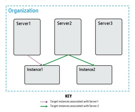
An Instance can be in multiple servers, but the servers must be in the same organization. For example, in the diagram Instance1 is associated with both Server1 and Server2.
