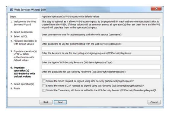
**Note:** If you set the values here, each operation will be assigned with the preset values. To change the value, you need to modify each flow in Studio or rerun the Web Services Wizard and select the **Overwrite the flow if already exists checkbox** in step 7.
