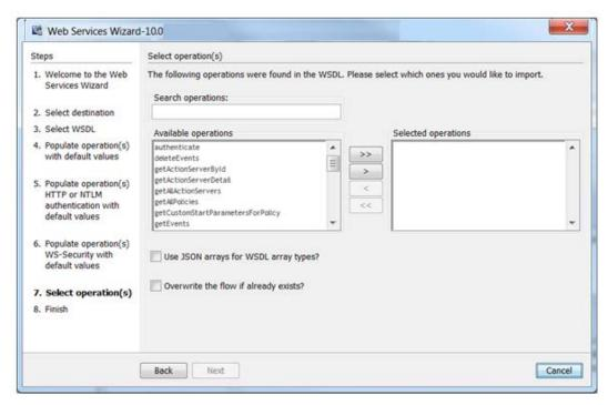
You can move the operations from one column to the other. Use the search textbox if the list is long, and you cannot find the required cmdlet. The wizard searches the list for the operations with names containing the search text. In addition, the wizard updates the list as you type.
