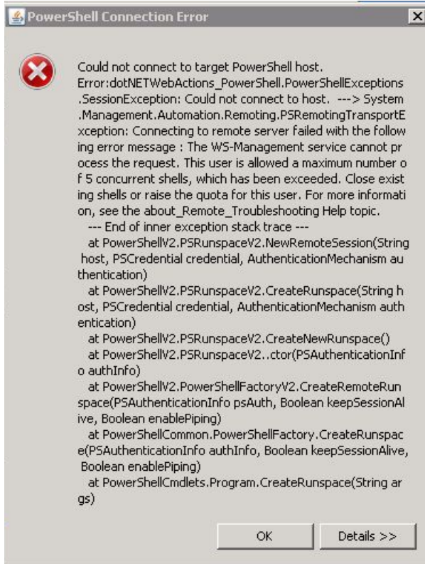
Figure 38: Connection Error - number of remote shells has been exceeded
