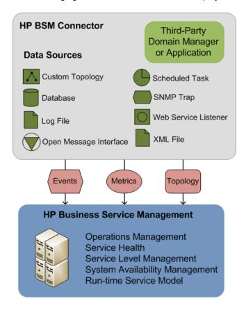
You typically install BSM Connector on the third-party system that acts as data source. For example, to integrate NNMi data into BSM, you install BSM Connector on the NNMi management server. However, BSM Connector can also access data sources on remote systems without the need to install data collectors on these systems.
