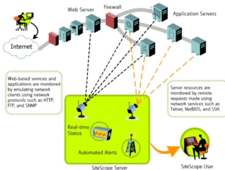
SiteScope Server monitors (for example, CPU, Disk Space, Memory, Service) can be used to monitor server resources on the following platforms:
