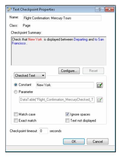
When **Checked Text** appears in the list box, the **Constant** field displays the text string you highlighted. This is the text UFT looks for when running the test.
