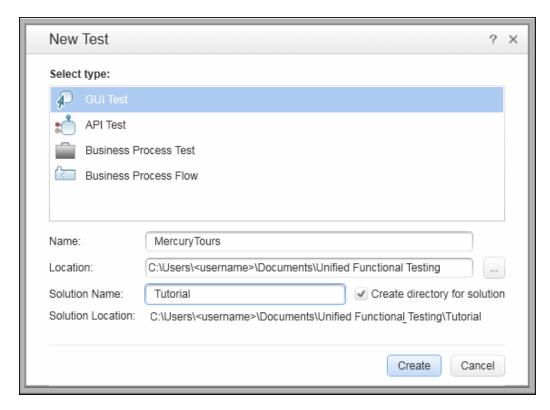
d. Click **Create.** A blank test opens, with the test flow displayed in the canvas, and a blank action tab opened in the background.
