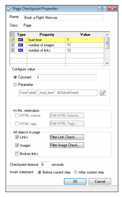
When you run the test, UFT checks the number of links and images in the page, and the load time, against those described in the table at the top of the dialog box. The page load time may vary from computer to computer and your load time results may not match the above image.
