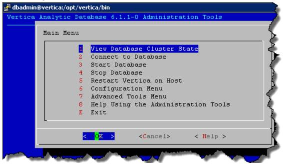
c. The opsadb database should have been created during the installation. Enter 1 to view the state of the database; then click **OK**. You should see a screen similar to the following if the opsadb database is running:
