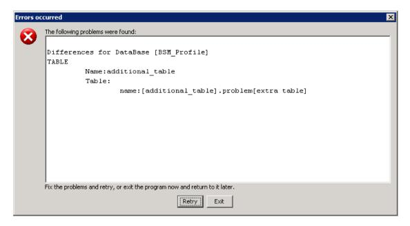
Either fix the problems found and click **Retry**, or click **Exit** and rerun the database schema verify program at a later date. A series of scripts, one for each problematic database, are created under **<BSM root directory>\dbverify\tmp**. If you are unable to fix the problems, contact HP Software Support for assistance.
