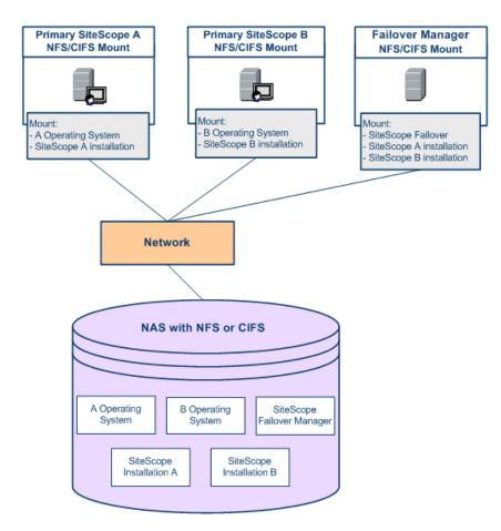
Primary SiteScope A and SiteScope Failover Manager mount the SiteScope A installation (logical volume) at the same moment.
