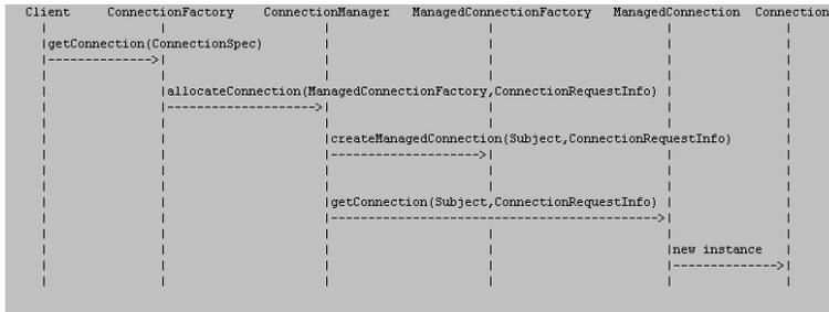
All implementations must return a **com.hp.ov.cit.connector.cci.Connection** type connection object.
