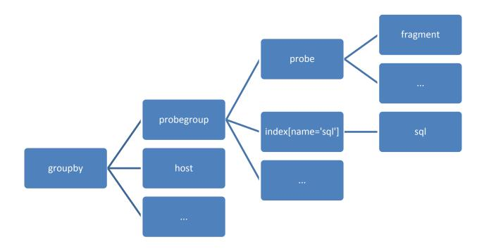
The root of the tree is always the groupby entity which allows Diagnostics to support multitenancy. Special "index" nodes don't have any metrics associated with them but act as a container to reduce the amount of nodes at the same level in the tree. For example, instead of putting all SQL statements (sql entity) directly under probegroup, the intermediary index entity groups all SQL statements under it, thus reducing the number of children under probegroup.
