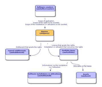
You will notice that there is no direct link between the counters and the objects that are counted. Queries are used to establish this link.
