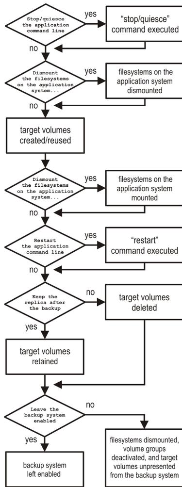
**Figure 11 ZDB-to-tape and ZDB-to-disk+tape session flow for filesystem backup objects**
