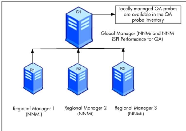
In this deployment scenario, only the locally managed QA probes are available in the QA probe inventory.
