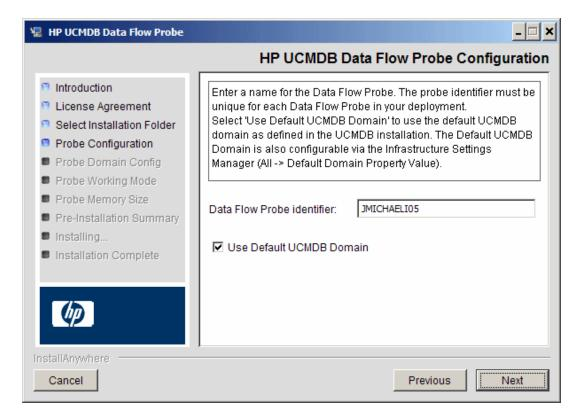
■ In the **Data Flow Probe Identifier** box, enter a name for the Probe that is used to identify it in your environment.
