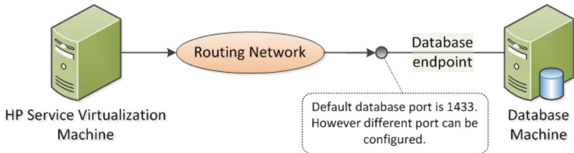
The default port of the database endpoint is **1433**. However, the database administrator can reconfigure the database to use a different port.
