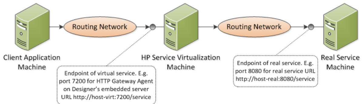
In this figure, the client application is reconfigured to communicate with the virtual service instead of the real service. The virtual service can be deployed on one of the following:
