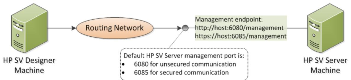
The Service Virtualization Designer also provides a management port, used mainly for connecting to integration testing tools.
