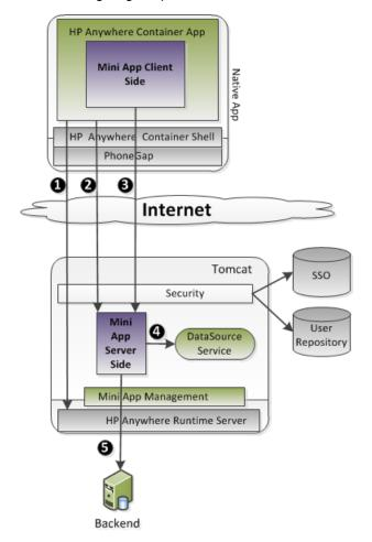
The HP Anywhere container application logs into the HP Anywhere runtime server using a security token. Authorization may be provided using SSO or basic authentication.
