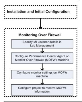
**Note:** Before you configure your system to monitor servers over a firewall, ensure that you have completed the configuration steps described in "Initial Configuration of the Over Firewall System" on page 199.
