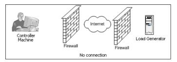
Performance Center solves this problem by using a communication configuration based on HTTPS or secured TCP/IP. This configuration uses the standard SSL port on the firewall (port 443). For more information on HTTPS and TCP/IP system configuration, see "Setting Up Your Deployment (TCP or HTTPS)" on page 200.
