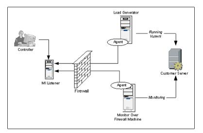
As explained in the previous section, the Performance Center agent is installed on both the Load Generator machine and the Monitor Over Firewall machine. During installation, the Performance Center agent is added as a Windows service.
