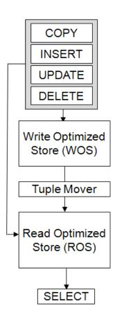
Write Optimized Store (WOS) is a memory-resident data structure for storing INSERT, UPDATE, DELETE, and COPY (without DIRECT hint) actions. Like the Read Optimized Store (ROS), the WOS is arranged by projection. To support very fast data load speeds, the WOS stores records without data compression or indexing. The WOS organizes data by epoch and holds both committed and uncommitted transaction data.
