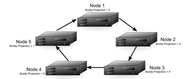
The diagram above shows a 5-node cluster that has a K-safety level of 1. Each of the nodes contains buddy projections for the data stored in the next higher node (node 1 has buddy projections for node 2, node 2 has buddy projections for node 3, etc.). Any of the nodes in the cluster could fail, and the database would still be able to continue running (although with lower performance, since one of the nodes has to handle its own workload and the workload of the failed node).
