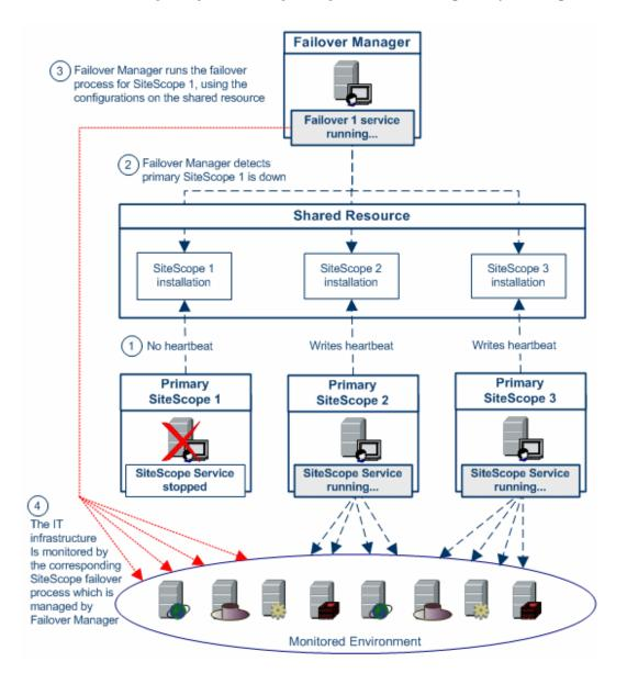
To support monitoring multiple primary SiteScopes from a single Failover machine, each primary SiteScope installation must be configured to answer on a unique port number. You can use the SiteScope Configuration Tool to view the full list of ports used by SiteScope, and to update the port numbers where necessary. For details, see "Using the SiteScope Configuration Tool" in the *HP SiteScope Deployment Guide* PDF.
