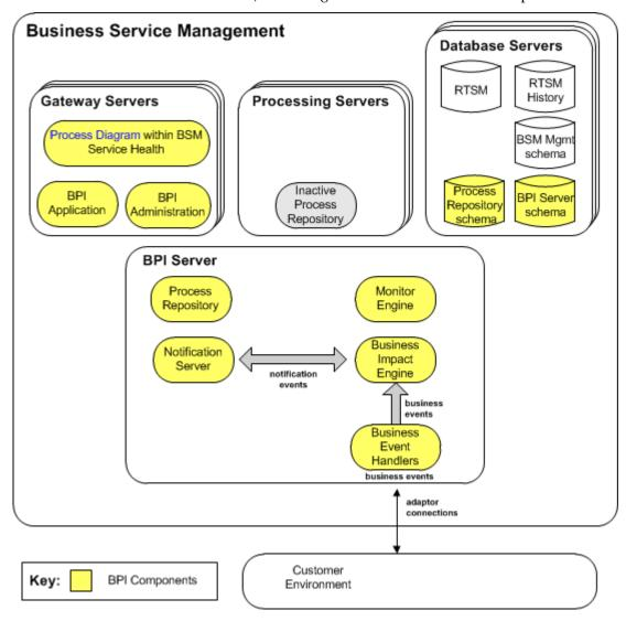
When you install the Server component of BPI, the existing Process Repository is replaced by a revised version, which is installed on the same system as the BPI Server. The revised Process Repository manages all Process Definitions from this point on, for processes that you create with instance tracking enabled and disabled.
