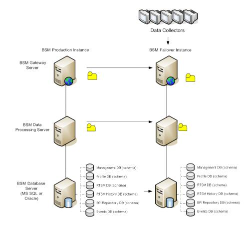
The following diagram shows a fully activated Failover instance:
