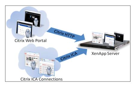
An end user starts by opening a Citrix Web portal and selecting one of the published applications. An ICA session is created, in which the selected application runs on the XenApp server, and the user uses the application remotely.
