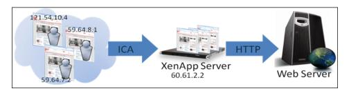
When monitoring the Web server with Real User Monitor, it is desirable to see the real end users as the clients, rather than having a single client combining all the traffic. To achieve such functionality, you must install the RUM HTTP Agent on the XenApp server.
