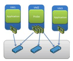
There are two entities in VMware—a virtual switch and portgroups. By default, a guest operating a system's virtual network adapter only receives frames specific for that adapter. Placing the guest adapter in promiscuous mode causes it to detect all frames passed through the virtual switch that are allowed under the VLAN policy for the associated portgroup.
