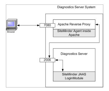
In the above diagram, an Apache web server listening for requests on port 7080 is configured as a reverse proxy. It contains the SiteMinder web agent which performs the authentication and if successful, allows Apache to pass the request through to port 2006 (or whatever Diagnostics Server port is configured) on which the Diagnostics server listens.
