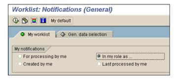
UFT uses the SAP GUI business component type (41) to identify the object as an SAPGuiRadioButton object. It creates an SAPGuiRadioButton test object with the name **In my role as...** and records the following properties and values as the description for the radio button.
