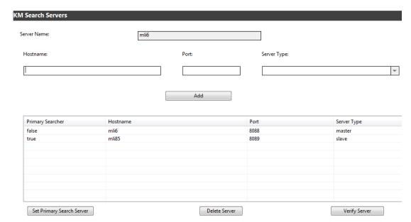
The following figure shows an example master and slave configuration.
