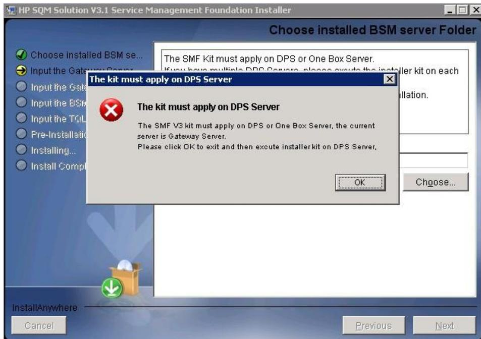
4. If the SMF 2.3 or above version is already installed, the following dialog box will appear, click ok to exit install application, and then uninstall the current exist SMF Kit before strating a new install.
