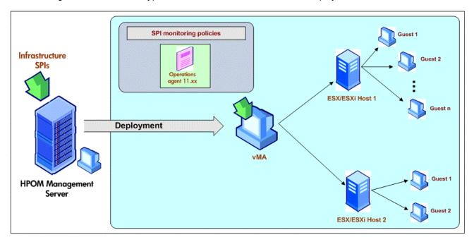
The following illustration shows a typical VMware environment with VI SPI deployed on a vMA:
