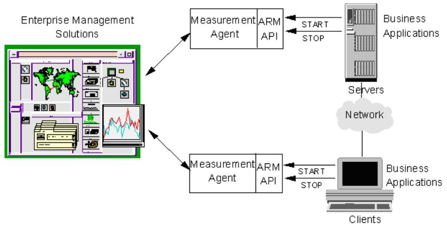
Figure 1 shows how enterprise management applications, measurement agents that implement the ARM API, and business applications that call the ARM API work together to provide a robust way to monitor application response.
